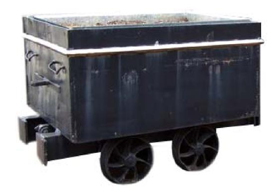
Next to the photo is a large cart. It is like the one in the photo! It is called a **coal cart**. It was used to move coal out of the mine. The coal cart moved on rails.
